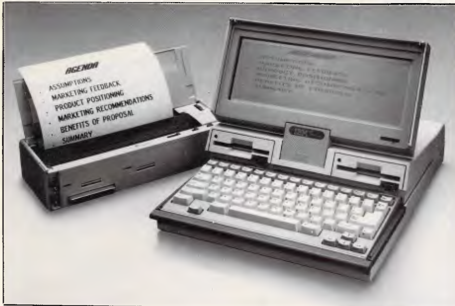
The Convertible's separate printer is a miniature thermal transfer unit
